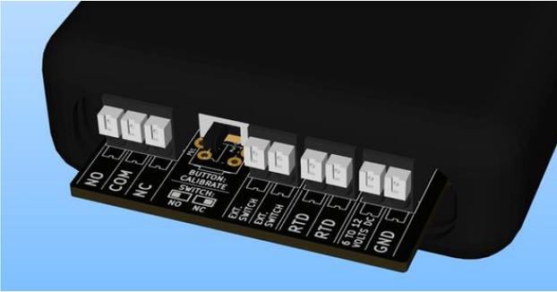
All external connections, and one slide switch, are on the bottom rear of the case, shown above.
